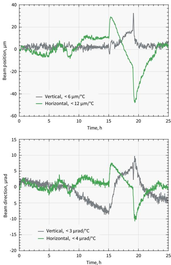
Output power, beam direction, and beam position of CARBIDE-CB5 under harsh environmental conditions
