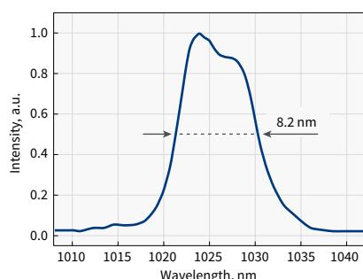
Typical spectrum of CARBIDE laser
