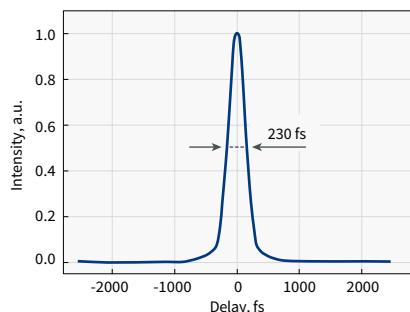
Typical pulse duration of CARBIDE laser
