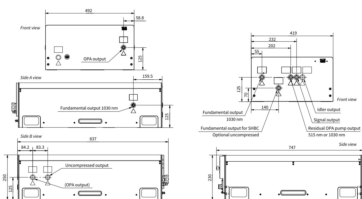
**Drawing and output ports of PHAROS-PH2 with fixed-wavelength I-OPA-FW-HP**
