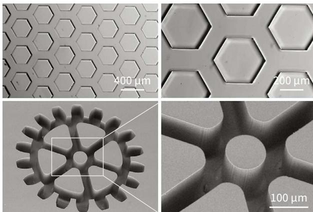
Various structures fabricated in fused silica glass.
