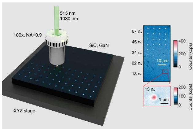
Illustration of the laser writing of color centers (left), silicon carbide containing arrays of laser-written color centers (right).
