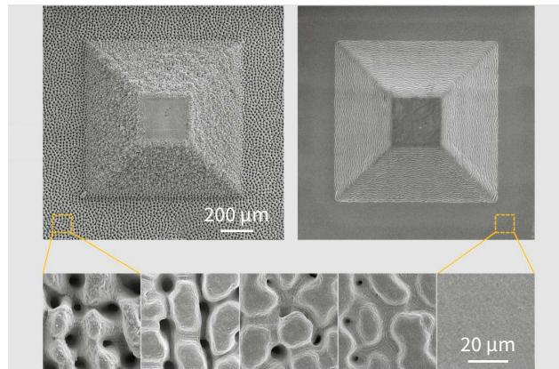
SEM image collage of structures ablated in stainless steel, before and after laser polishing using GHz burst mode (from left to right).
