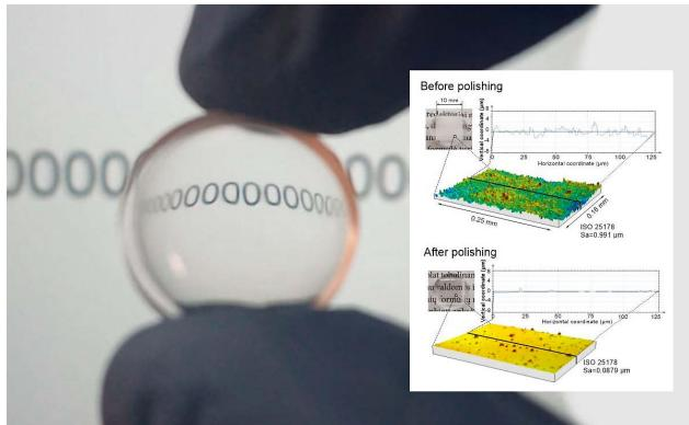
Polished curved surface and surface roughness measurements before and after polishing with GHz BiBurst.
