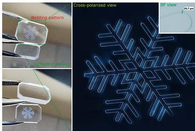
Example of 1 mm thick fused silica glass welding.
