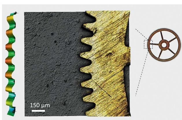
Example of gear cut from brass. Source: Lasea.
