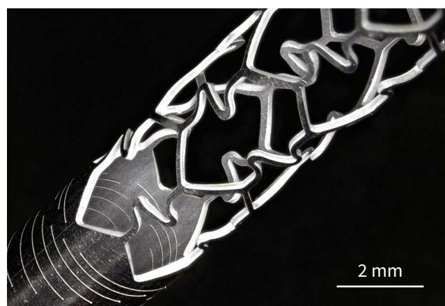
Stent cut using CARBIDE laser.
