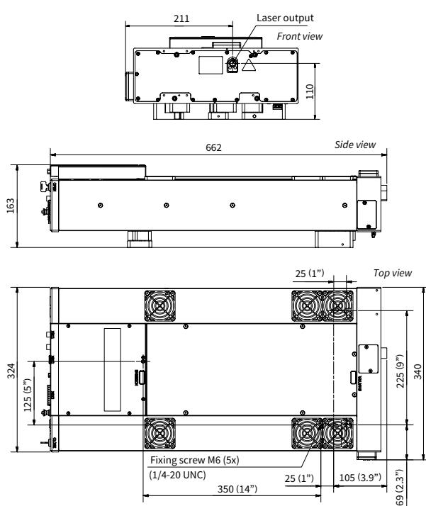
Drawing of air-cooled CARBIDE-CB5 with attenuator
