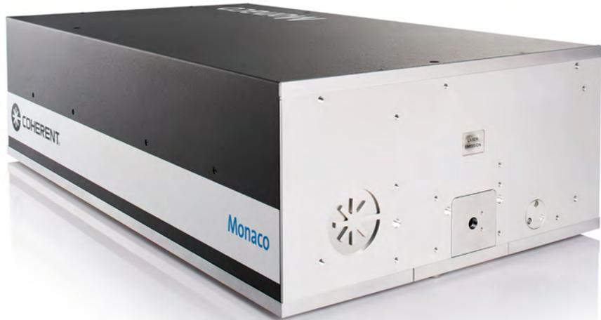
Monaco is a diode-pumped, fiber-based, Chirped Pulse Amplifier (CPA) MOPA architecture designed for heavy-use, 24/7 applications. The fiber based design offers energy and repetition rate diversity required to cover a wide range of applications requiring high repetition rate, energetic femto-second pulses.
